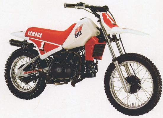
Powered by Yamaha's tried-and-true 2-stroke reed-valve engine, this child's size fun-bike features everything you'd expect: fully automatic transmission, shaft drive, telescopic front forks, dual rear shock absorbers, hand-operated front and rear brakes and a weight of only 37kg.
