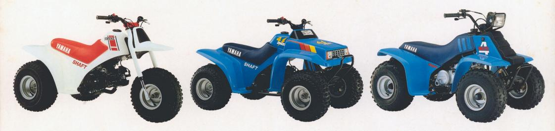
The YT60 downsizes the virtues of Yamaha Tri-Motos for first-timers. The 59cc 2-stroke engine delivers plenty of pep through its automatic transmission. The shaft drive and CD ignition help eliminate maintenance. And the trio of fat, corded tyres provide plenty of traction with stability. Once you get your kid on the YT60, maybe one of the biggest problems will be getting him off.
