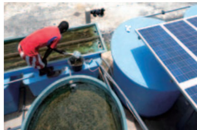
With no need for filters or coagulant chemicals, maintenance is easy and does not require specialists
