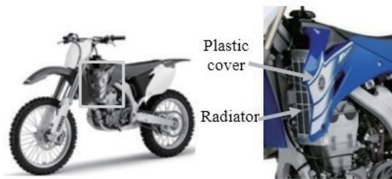
Figure 1: Appearance of radiator and plastic cover
