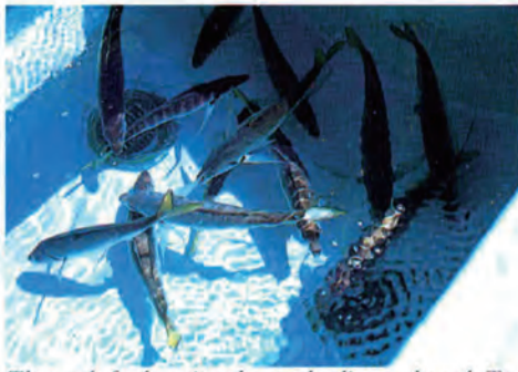
The tank for keeping the catch alive on board. To prevent the water from sloshing around violently when the boat is in motion, a lid made of netting material is placed over the scupper.
