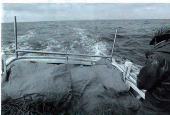
The net laying operation. The net, arranged in order on the aft deck the day before, is fed into the sea while running ahead at full speed.
