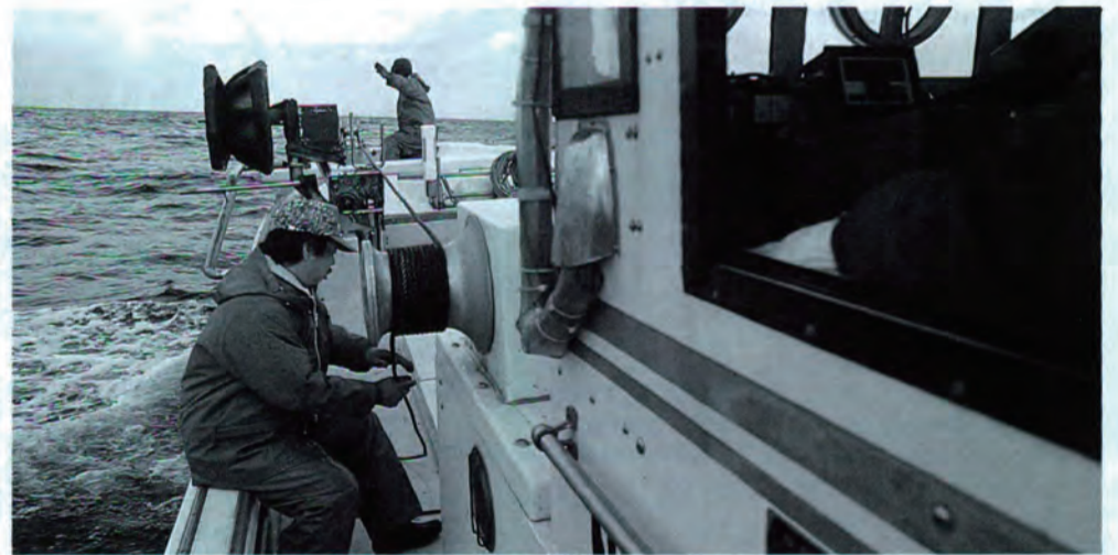
The net rope is pulled in by a side roller run directly off the main engine.
