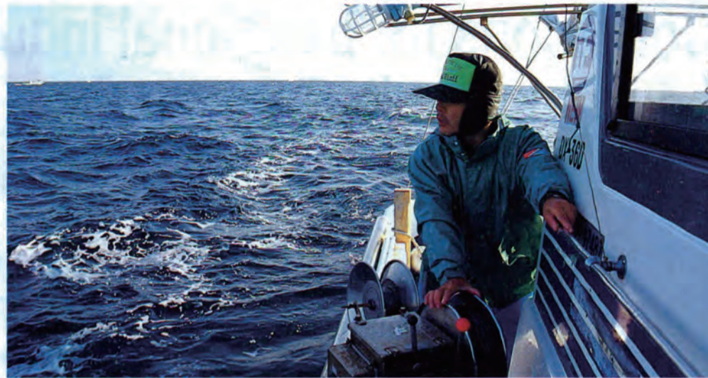
The trolling operation. After the line has been completely fed into the water, the boat proceeds to troll slowly for about 30 minutes before hauling in the main line by means of a line hauler.
