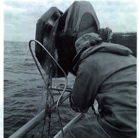
The net hauler (made of hardened plastic) and a stainless steel pipe guide to help guide the net into the hauler.
