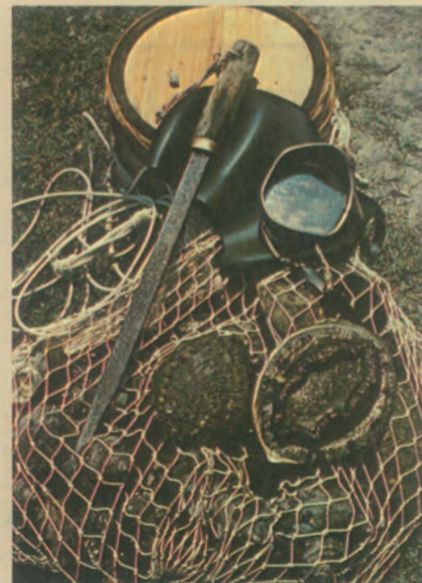
Detaching abalone from the rocks they adhere to is difficult with just the bare hand. Divers take along a steel spatula to pry the abalone loose, taking advantage of a lever action. Depending on the makeup of the reef, they may use a variety of spatulas ranging in length from about 20cm to 60cm.
