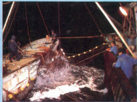
The bunt is hauled in by hands with the aid of side-roller.
