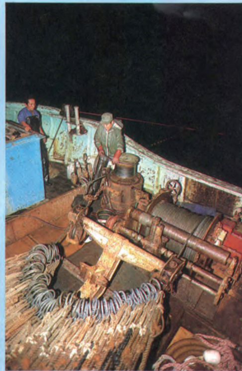
Purse line is hauled in by purse wire winch.
