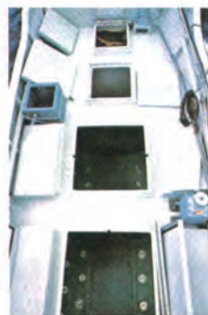
Live fish tank at the fore deck (equipped with a water sprinkler).
