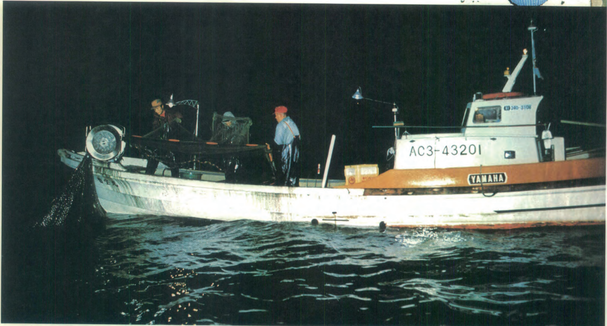
Net hauling (a hauler is used to pull up a net while a searchlight is shown on the water surface)
